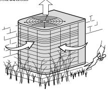
to work harder and use more energy. Keep shrubbery trimmed away from the unit and periodically check for debris which may have collected around the unit.
